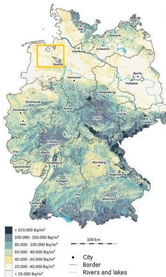
Fig. 2 Map of Germany with the average radon concentrations in the soil air showing the section depicted in Fig. 4. Map according to [19] amended and supplemented by the author
