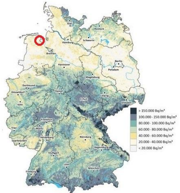
Fig. 6 Radon in the ground, map of Germany from [11], modified by the author, marked the town of Wilhelmshaven.
