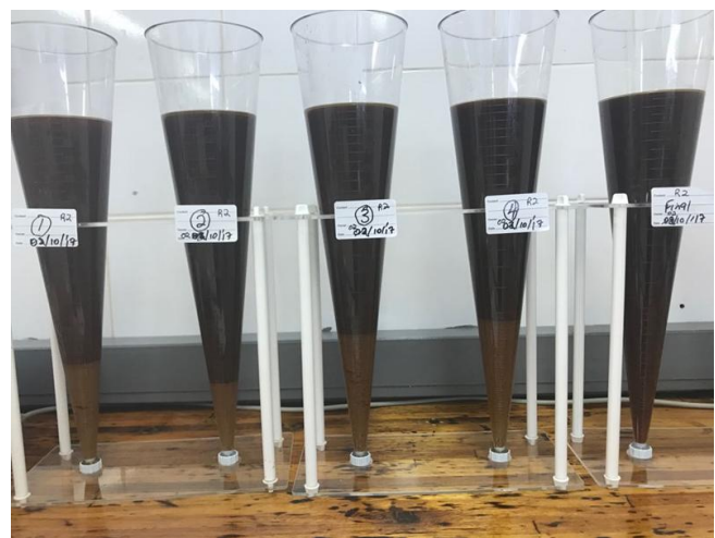
Fig. 4 Determination of settleable suspended solids in baker's yeast effluent
