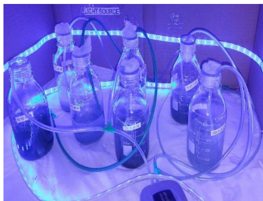
Fig. 1 1 L reactor vessels used for microalgae cultivation
