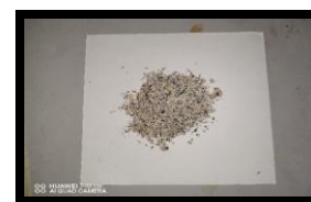
Fig. 2(d) Crushed castor seed after solvent extraction and drying
