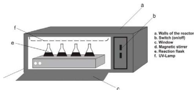
Fig. 2 Photoreactor equipped with a 40 Watt UV lamp and a series of magnetic stirrers [12]
