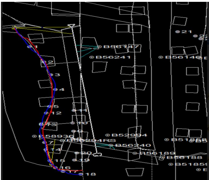
Fig. 7 KL33 16 08S showing underground face that was measured by tapes and also measured by Total station.
