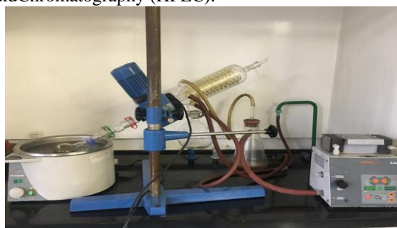
Fig. 2 Rotary evaporator with a sample being separated in terms of their relative boiling points.
