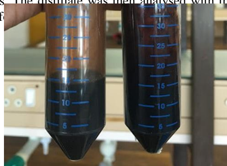
Fig.5 Mixture from Parr reactor prior filtration, depicting the dark colour and viscosity of the mixture.
