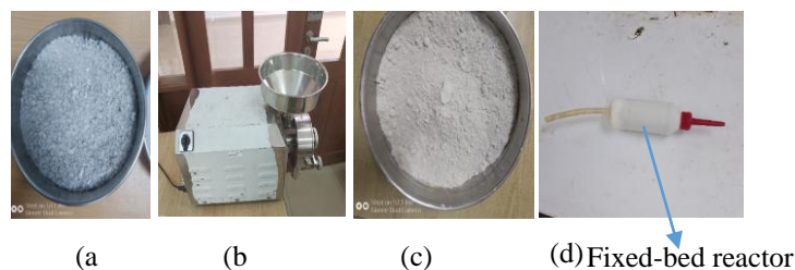
Fig 1: Preparation of sodium carbonate sorbent for sorption purposes: (a) bigger particle size (b) grinding machine (c) working size (d) Fixed bed column.
