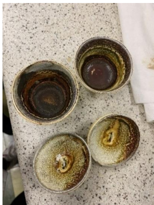
Fig. 4. Photo of melted \text{Na}_2\text{SO}_4 when heated to 1000 °C
