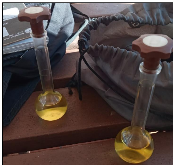
Fig 6. Solution generated from the digestion of the electrode materials in aqua regia .
