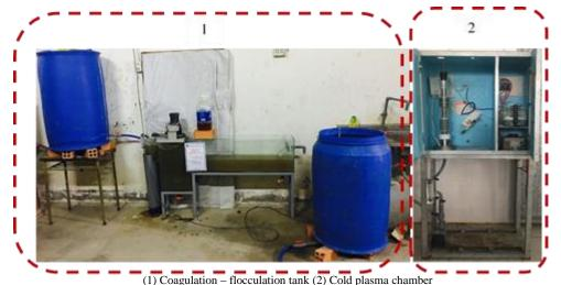
Fig. 1: Lab-scale treatment model of wastewater from snakehead fish lined tank
