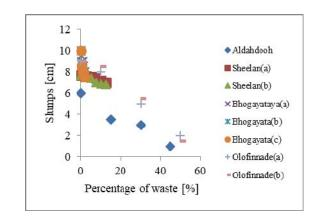
Fig. 1: Variation of slumps in referenced tests.
