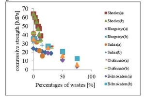
Fig. 3: Variation of compressive strengths in referenced tests.
