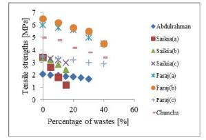
Fig.4: Variation of tensile strengths in referenced tests
