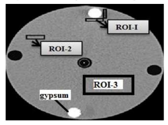
Fig. 2 Regions of interest (ROIs-1 and ROI-2) were used for beam hardening artifact assessment. Regionsof interest (ROI-3) was used to measure the standard deviation (Image noise measurements)
