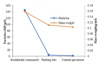
Fig. 3. Characteristics of microplastics distribution in urban runoff
