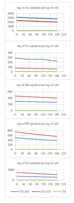
Fig. 2 Reduction of elements in contaminated soils after 180 days of phytoremediation
