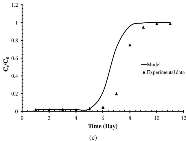
Fig. 3. Linear plot of Thomas model with experimental data. (a) Bungor soil (b) Bungor soil with DPL and (c) Bungor soil with *R. palustris* adhered on DPL
