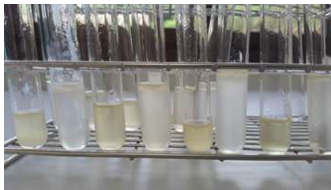
Fig.1 Top (PEG 3350) and bottom (K-citrate) phases from the aqueous two phase system
