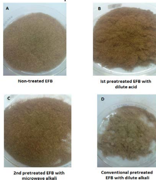
Fig. 1. Morphologies of the EFB samples (A) the non-treated EFB (B) the first dilute acid-pretreated EFB (C) the second sequential acid/alkali- pretreated EPFB fiber (D) Conventional dilute alkali pretreated EFB
