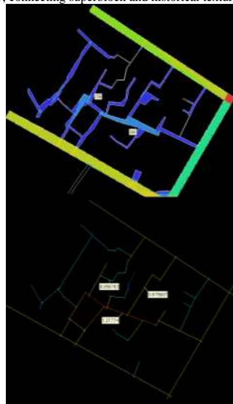
Fig.11: VGA analysis (up), Spatial integration analysis (down) of the area.
