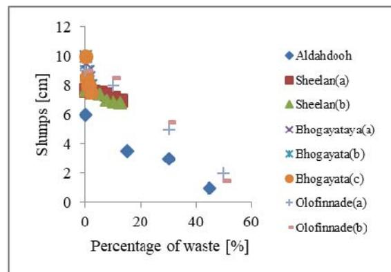
Fig. 1: Variation of slumps in referenced tests.
