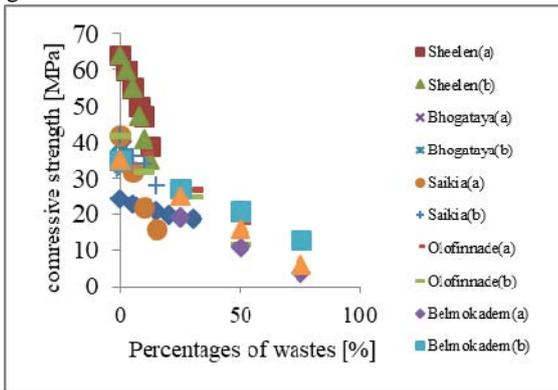
Fig. 3: Variation of compressive strengths in referenced tests.
