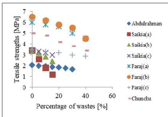
Fig.4: Variation of tensile strengths in referenced tests
