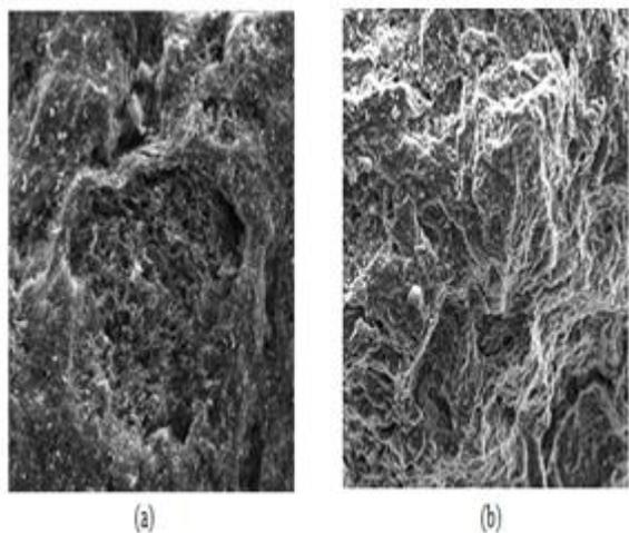
Figure 3: Scanning Electron Micrographs of the GAC before (a) and after (b) adsorption process
