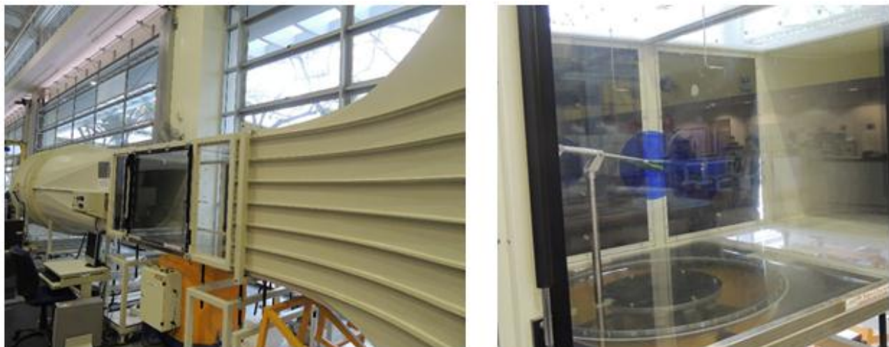
Fig.5: Wind tunnel testing of NTU-20-V airfoil in the wind tunnel.
