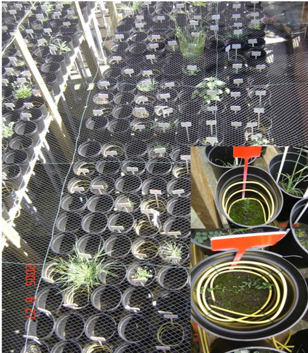
Fig. 1. Heating cables used in the experiment to elevate temperature by 3 °C above ambient within the pot. (MATERIAL AND METHODS: PLANT MATERIAL AND EXPERIMENTAL DESIGN)
