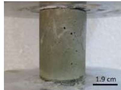
Fig. 4. BFRC during compression test
