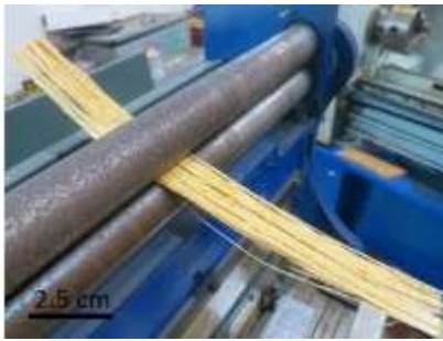
Fig. 1. Bamboo fibers being fed into a rolling machine
