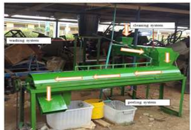
Plate 2: The complete machine assembly showing the direction of cassava flow
