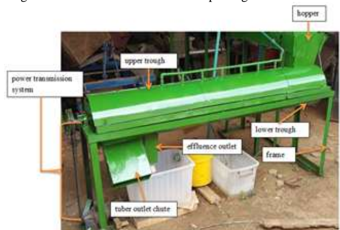
Plate 1: The peeling Unit of the Cleaning, Peeling and Washing Machine for Cassava Tubers
