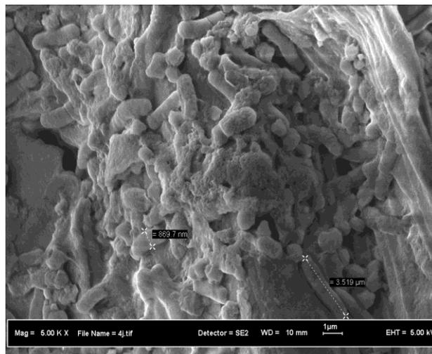
Fig. 2 FESEM image of DPL adhered with *R. palustris* bacterium (rod-shaped structures). The number of colony forming unit (CFU) of *R. palustris* used in this experiment was  $6 \times 10^7$  which was freshly prepared.
